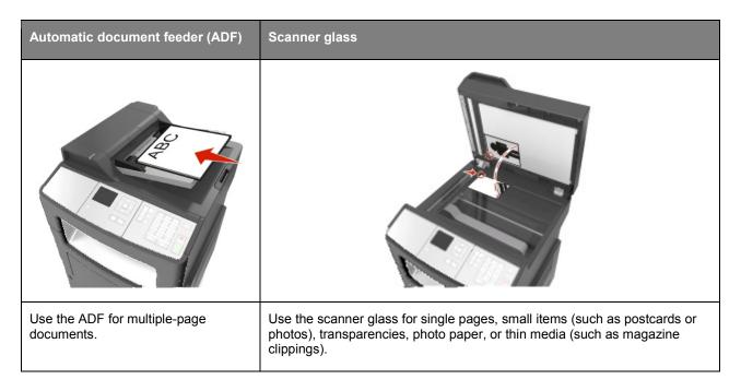
The scanner lets you scan documents directly to a computer. The computer does not have to be directly connected to the printer for you to receive Scan to PC images. You can scan the document back to the computer over the network by creating a scan profile on the computer and then downloading the profile to the printer.
