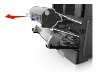
3. Lift the blue handle, and then pull the imaging unit out of the printer.
