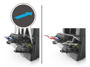
7. Insert the toner cartridge into the printer by aligning the side rails of the cartridge with the arrows on the side rails inside the printer.
