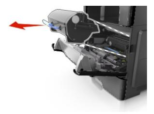
3. Lift the blue handle, and then pull the imaging unit out of the printer.
