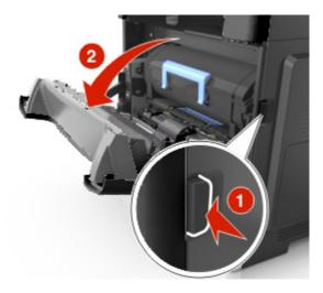
2. Pull the toner cartridge out using the handle.
